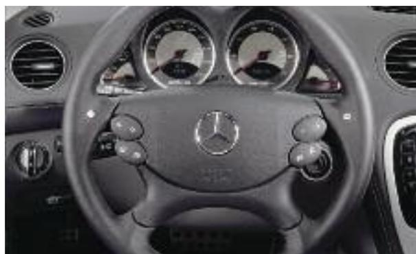
Gear controls on steering wheel
