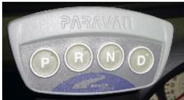
Electronic gear selector, from Adaptacar
