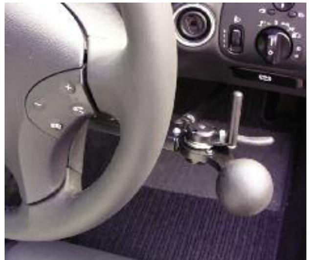
*Brig Ayd Trigger control. Pull trigger to accelerate (electronic), push away to brake*
