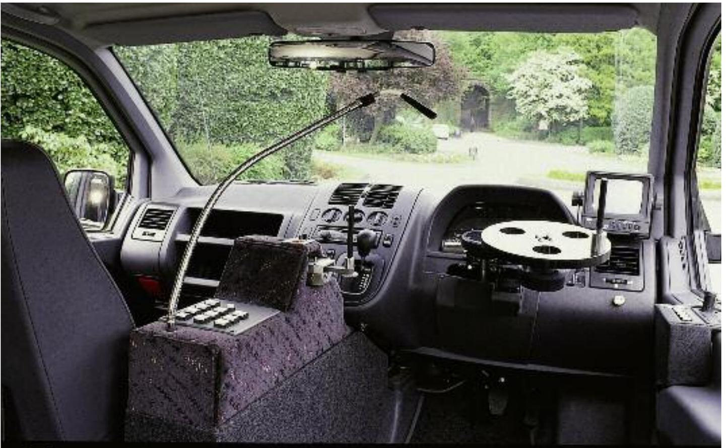
*Drive from wheelchair vehicle with horizontal steering wheel, joystick speed control suck and blow tube for secondary controls and reversing camera*
