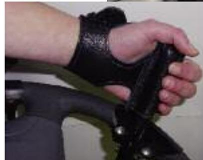
The glove has a sleeve that fits over a peg on the steering wheel
