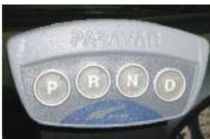
*Spacedrive push-button gear selector – Adaptacar*
