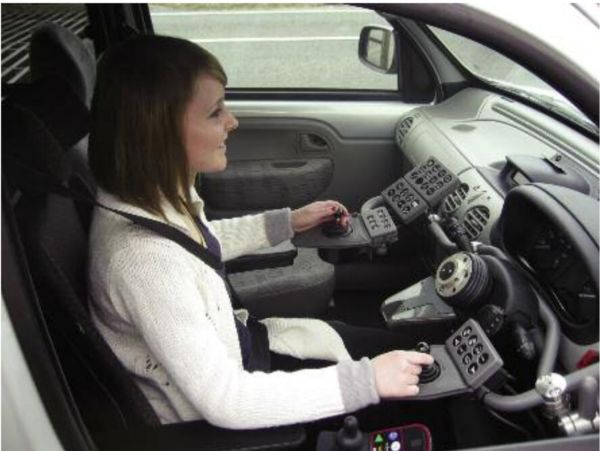
*Drive from wheelchair vehicle with joystick steering and speed control; keypads for gears and secondary controls*
