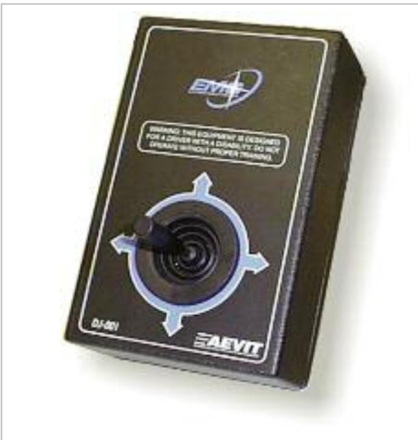
*This AEVIT J control from D S & P is used to steer, brake and accelerate. It can be placed in any position which suits you. You push the joystick from side to side to steer, pull it back to accelerate and push it forwards to brake. It has speed sensitive steering, which adjusts the action and feel of the joystick to your speed. This makes parking and manoeuvring easier. You can switch the system off if someone else is driving*
